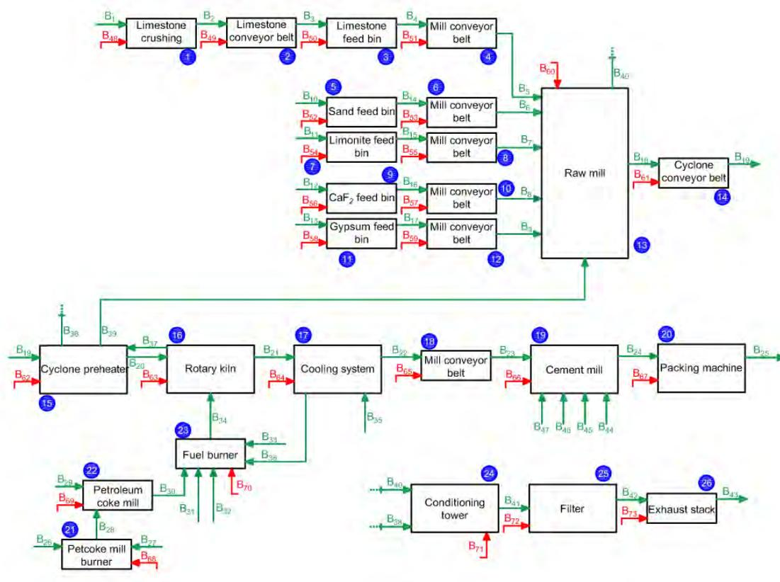
**Figure 1.** Process flow diagram of the studied cement plant.
